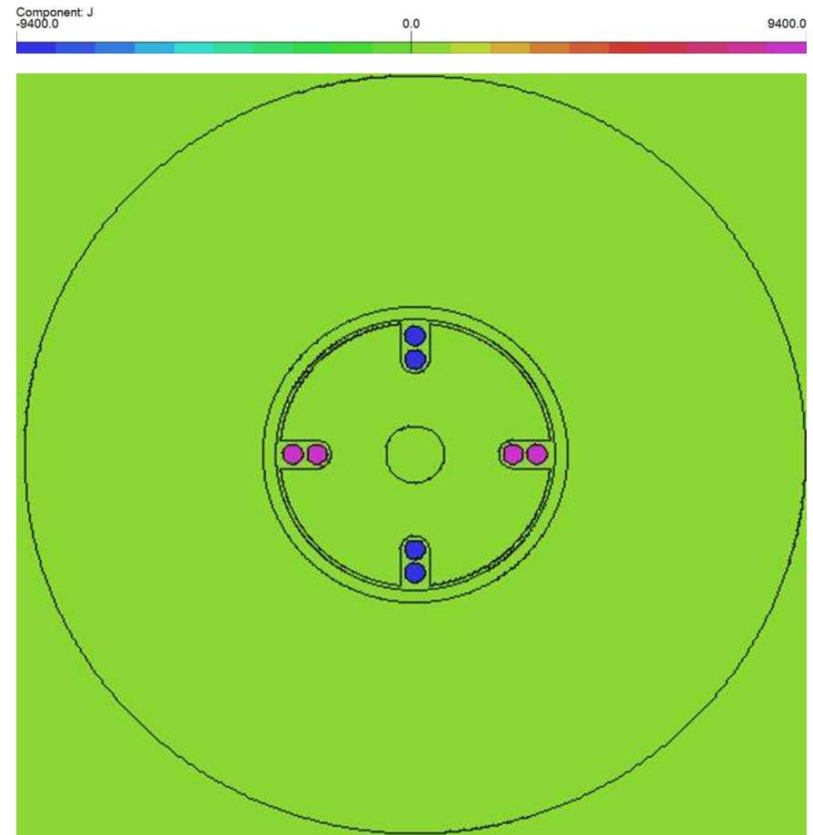
Current density plot @ peak magnetizing current
